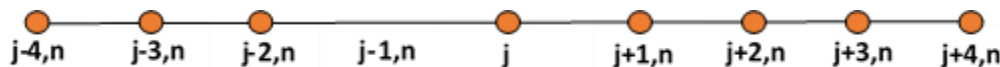
Figure 38 – One dimensional space divided into evenly spaced segments, where j is taken to be the center point. The variable j represents the spatial coordinate and n represents the temporal step.
